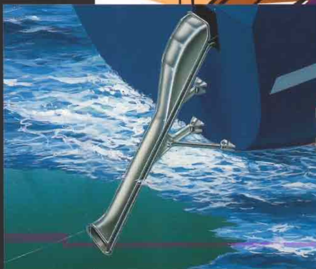
A funnel developed by O. Mustad & Son A.S. for underwater setting of longline astern of the vessel
