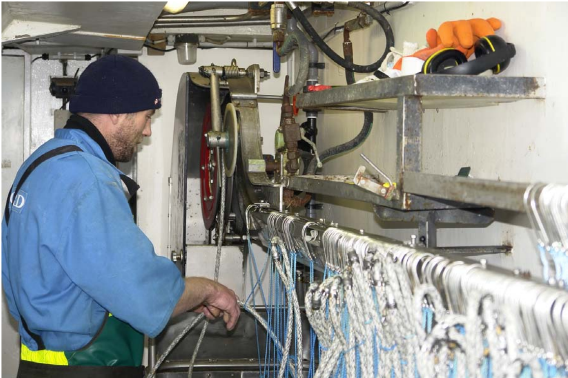
Figure 4. Combi (Combination hauler/hook separator).
