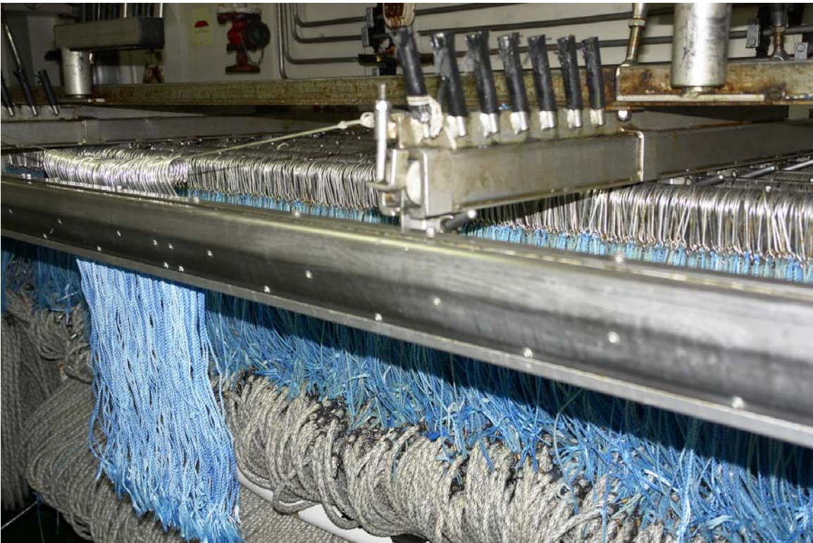
Figure 6. Loaded magazines with spare hooks and snoods in the foreground.
