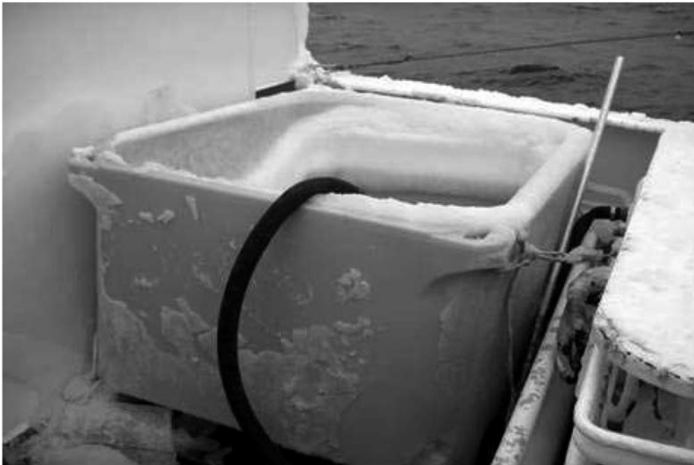
Figure 2: Experimental tanks used on the Viking Bay . The exposed position, lack of lid and lack of flow-through water led to the water freezing on several occasions.
