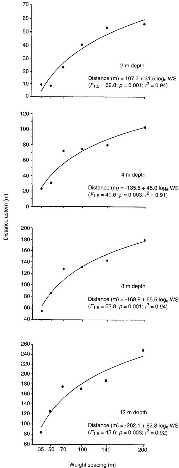
Figure 5: Longline distance astern from water entry point (15 m behind vessel) at depths, shown as a function of weight spacing (WS in metres) on longline set by the *CFL Pioneer*. Results for 2 m depth are provisional. Ship setting speed was 2.572 m/s (5 knots). Closed circles represent means from three dive recorders.
