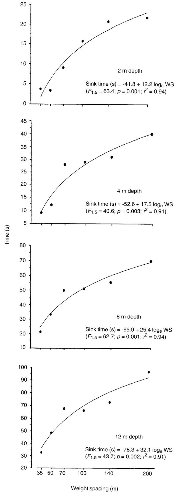
Figure 4: Longline sink time (seconds) to depth, shown as a function of weight spacing (WS in metres) on longline set by the CFL *Pioneer*. Results for 2 m depth are provisional (see text). Note variation in increments on 'y' axes. Closed circles represent means from three dive recorders.
