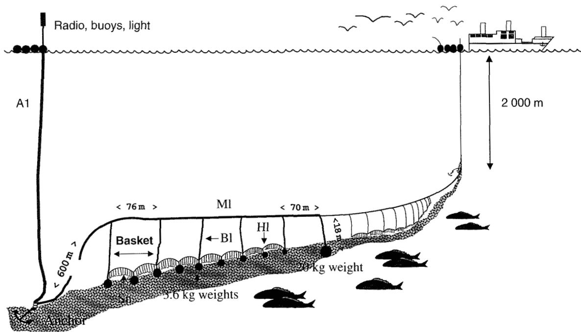
Figure 2: Longline configuration of the *In Sung 66* (Spanish system, double line) used for toothfish fishing. Anchor lines (A1), mother line (M1), branch lines (B1), hook line (H1) and snood lines (Sn) are 20, 18, 9, 5 and 2.5–3 mm in diameter respectively. Baited hooks are deployed in 'baskets', with each basket containing 76 m of hook line and 48 baited hooks.
