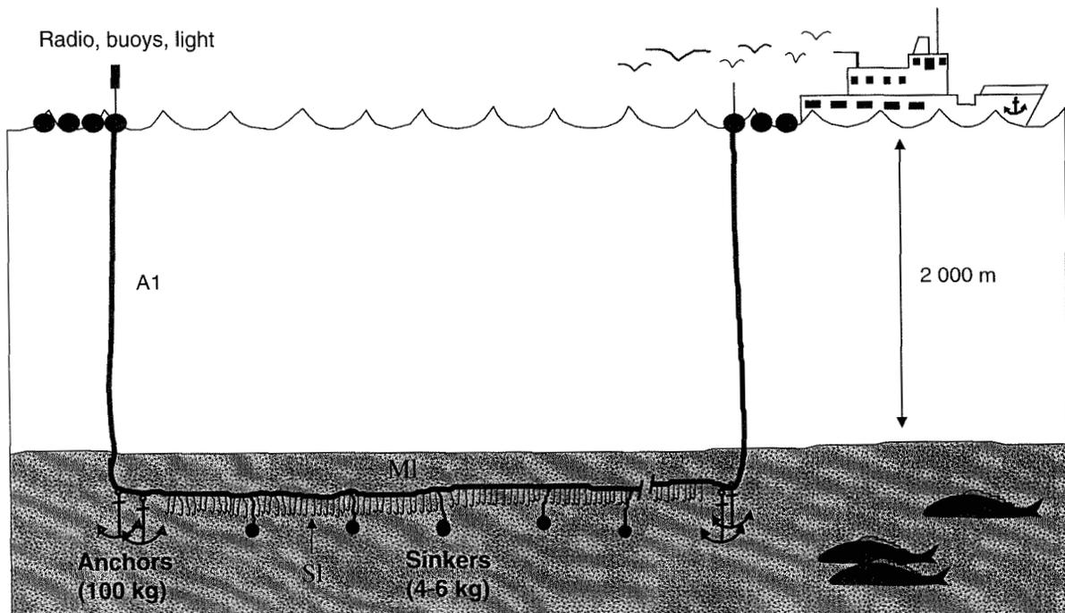
Figure 1: Longline configuration of the *CFL Pioneer* (Mustad autoline (single line) method) used for toothfish fishing. Anchor lines (A1), mother line (M1) and snood line (Sn) are 18, 11.5 and 3 mm in diameter respectively.
